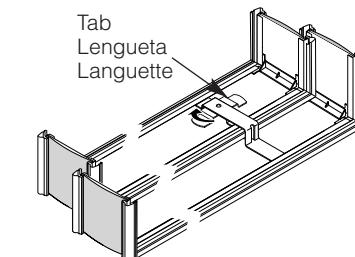
Rotate tab at bottom of valance bracket 90°, fitting it into the bottom valance channel. Space brackets equally.
