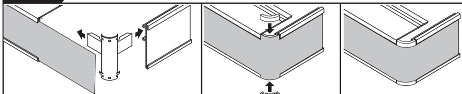
Insert valance corner into channels of valance and return; attach corner caps.
