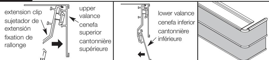
Attach double valance extension clips to channel of upper valance and returns; snap lower valance onto extension clips.
