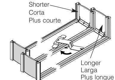
Lay shorter valance on top of longer valance. Insert double valance bracket into longer valance channels and turn until perpendicular to valance.
