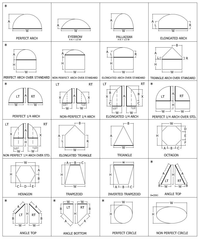
NOTE: TO DETERMINE "X" MEASUREMENT DIVIDE "W" IN HALF - MEASURE FROM THIS POINT STRAIGHT UP (PLUMB) AS SHOWN IN DIAGRAM. NOTE: \* NO TEMPLATE REQUIRED
